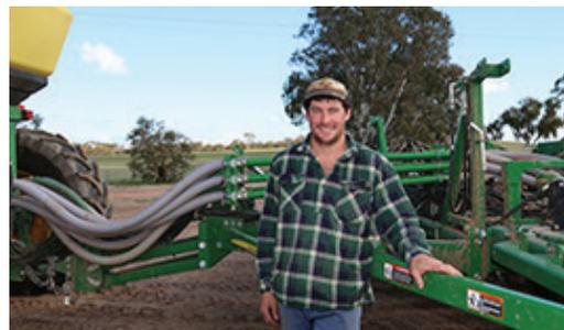
Featured growers Glenn Smith and Jess Edmonds upgraded from an older Flexi-Coil spring tyne seeding bar to a John Deere Conserver Pak precision seeder, which is 17 metres (56 foot) in width, uses 12-inch single row spacings for lupins and canola and paired row splitter boots for the cereals - which gives them a nine, a three and a nine-inch split.
